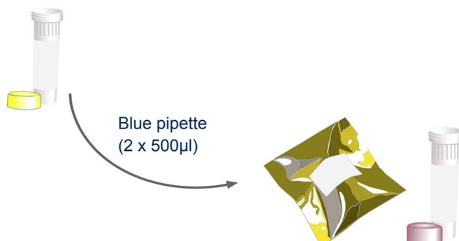
Use the blue pipette to transfer 1000µl (2 x 500µl) of template preparation buffer into the positive control template tube. Cap and shake tube to mix.
