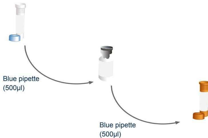
Use the blue pipette to transfer 500µl\* of the oasis Master Mix resuspension buffer into the tube of lyophilised oasis Master Mix and mix well by gently swirling. Then transfer all of that master mix into the brown tube labelled E.coli\_O157 primers/probe.
