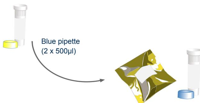
Use the blue pipette to transfer 1000 $\mu$ l (2 x 500 $\mu$ l) of template preparation buffer into the Internal Extraction Control DNA tube. Cap and shake tube to mix.
