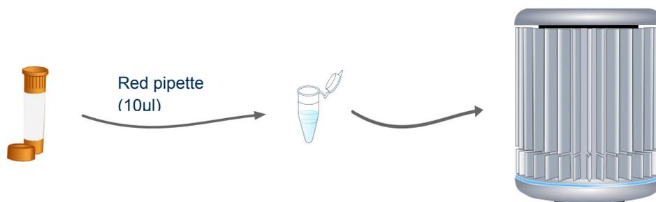
For every reaction to be run, use the red pipette to add 10 $\mu$ l of your E.coli\_O157 reaction mix to every tube.
