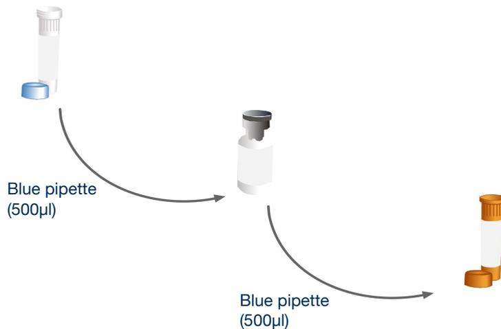
Use the blue pipette to transfer 500µl\* of the oasis Master Mix resuspension buffer into the tube of lyophilised oasis Master Mix and mix well by gently swirling. Then transfer all of that master mix into the brown tube labelled Sheep primers/probe.
