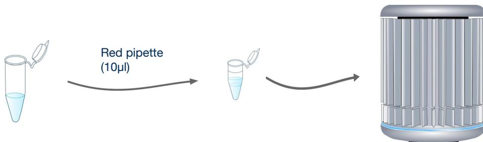
For each sample you wish to analyse, use the red pipette to add 10µl of your DNA sample to the required reaction tubes. Close these tubes after adding the sample. Always change pipette tips between samples.
