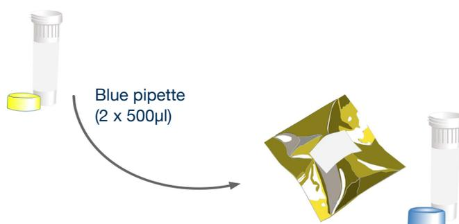
Use the blue pipette to transfer 1000µl (2 x 500µl) of template preparation buffer into the Internal Extraction Control DNA tube. Cap and shake tube to mix.
