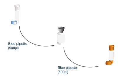
Use the blue pipette to transfer 500µl\* of the oasig Master Mix resuspension buffer into the tube of lyophilised oasig Master Mix and mix well by gently swirling. Then transfer all of that master mix into the brown tube labelled Y.pestis primers/probe.
