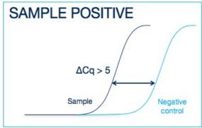
If the sample amplifies > 5 Cq earlier than the negative control then the sample should be reinterpreted (via the table above) with the negative control verified as negative. INCONCLUSIVE
