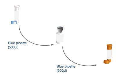
Use the blue pipette to transfer 500µl\* of the oasig Master Mix resuspension buffer into the tube of lyophilised oasig Master Mix and mix well by gently swirling. Then transfer all of that master mix into the brown tube labelled P.vivax primers/probe.
