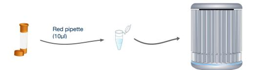
For every reaction to be run, use the red pipette to add 10µl of your P.vivax reaction mix to every tube.
