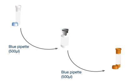
Use the blue pipette to transfer 500µl\* of the oasig Master Mix resuspension buffer into the tube of lyophilised oasig Master Mix and mix well by gently swirling. Then transfer all of that master mix into the brown tube labelled P.acnes primers/probe.
