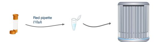
For every reaction to be run, use the red pipette to add  $10\mu$ I of your P.acnes reaction mix to every tube.
