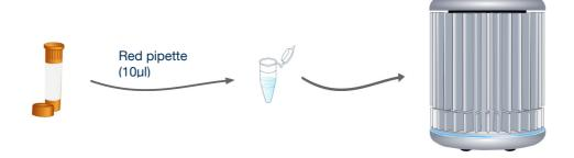
For every reaction to be run, use the red pipette to add 10µl of your E.faecalis reaction mix to every tube.
