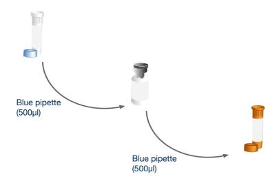
Use the blue pipette to transfer 500µl\* of the oasig Master Mix resuspension buffer into the tube of lyophilised oasig Master Mix and mix well by gently swirling. Then transfer all of that master mix into the brown tube labelled AIDV primers/probe.
