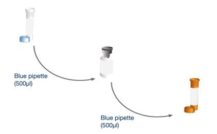
Use the blue pipette to transfer 500µl\* of the oasig Master Mix resuspension buffer into the tube of lyophilised oasig Master Mix and mix well by gently swirling. Then transfer all of that master mix into the brown tube labelled T.cruzi primers/probe.
