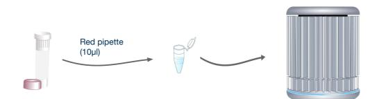
Take great care when setting up your positive control. The positive control template has the potential to give you a false positive signal in your other samples. Set positive controls up last after all other sample tubes are closed. Always change pipette tips between samples. You may even choose to set up positive controls in a separate room.
