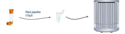
For every reaction to be run, use the red pipette to add 10µl of your M.pneumoniae reaction mix to every tube.
