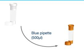
Then use the blue pipette to transfer 500µl of water into the brown tube labelled ISAV-CA primers/probe. Cap and shake tube to mix. A thorough shake is essential to ensure that all components are resuspended. **Failure to mix well can produce poor kit performance.**
