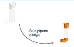
Then use the blue pipette to transfer 500µl of water into the brown tube labelled Human Rotavirus A primers/probe. Cap and shake tube to mix. A thorough shake is essential to ensure that all components are resuspended. Failure to mix well can produce poor kit performance.
