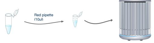
For each sample you wish to analyse, use the red pipette to add 10µl of your DNA sample to the required reaction tubes. Close these tubes after adding the sample. Always change pipette tips between samples.
