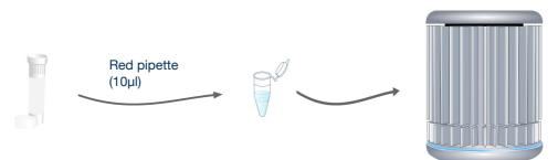
For each test you will require a negative control. Instead of DNA, water is used. This sample should typically prove negative thus proving that all of your positive samples really are positive.
