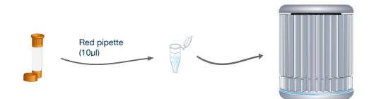
For every reaction to be run, use the red pipette to add 10µl of your E.faecium reaction mix to every tube.
