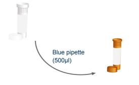
Then use the blue pipette to transfer 500µl of water into the brown tube labelled Dengue primers/probe. Cap and shake tube to mix. A thorough shake is essential to ensure that all components are resuspended. **Failure to mix well can produce poor kit performance.**
