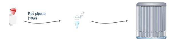
For every reaction to be run, use the red pipette to add 10µl of the oasig OneStep Master Mix to the tubes containing primer/probe mix.
