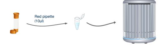
For every reaction to be run, use the red pipette to add 10µl of your BPV reaction mix to every tube.
